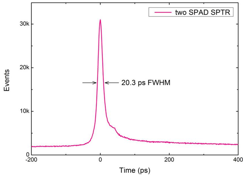
Figure 2. The TCSPC measurement provides the number of events over the measured photon arrival time difference. The FWHM is a measure for the timing resolution of the entire system.
