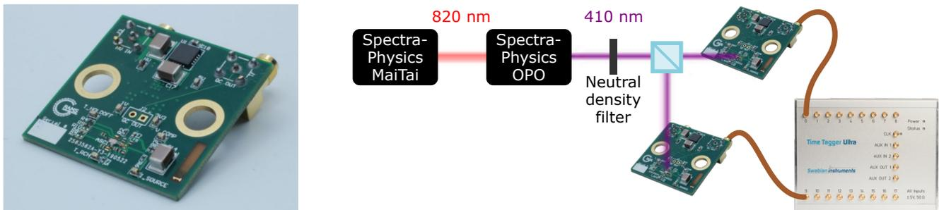
Figure 1. The SPAD detector provided by Sherbrooke University and a scheme of the setup. The setup consist of a Spectra Physics Mai Tai 80 MHz Ti:Sapphire femtosecond pulsed laser and a Spectra-Physics Inspire optical parametric oscillator (OPO) and a pre-release unit of the new Time Tagger Ultra HiRes.
